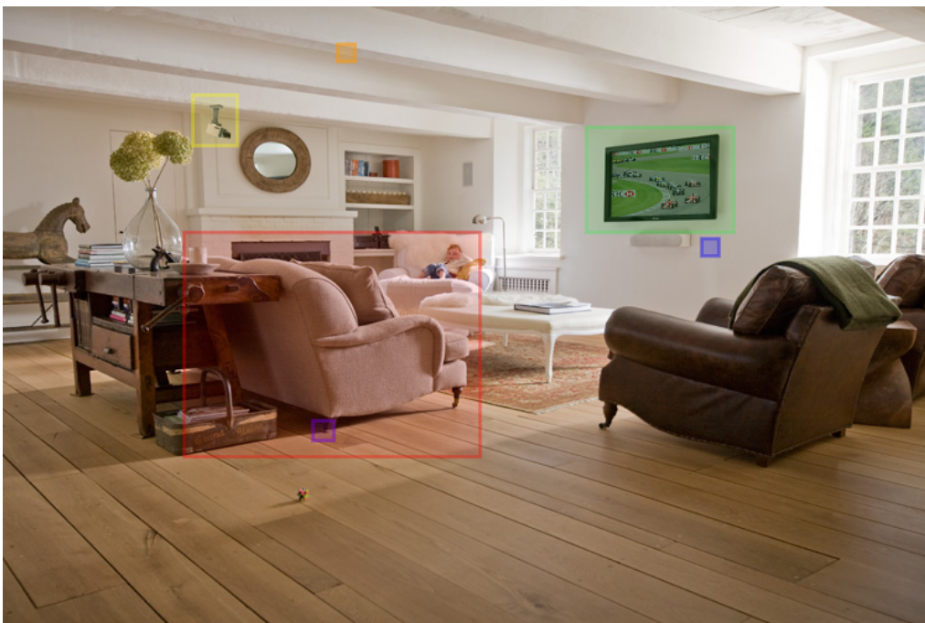
Figuur 3.2: Situation overview: Red - Hotspot A, Green - Hotspot C, Yellow - Camera, Orange - Ambient light sensor, Blue - TV light sensor, Purple - Pressure sensor
